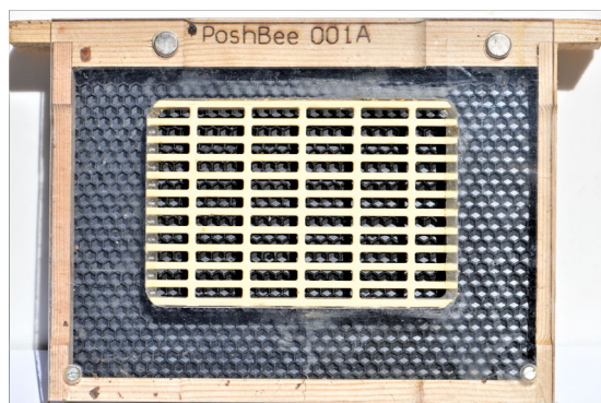
Figure 1. The Study Frame showing the black plastic foundation and the removable queen excluder/ acrylic cover.
